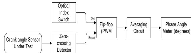
Figure 2: Test fixture block diagram
